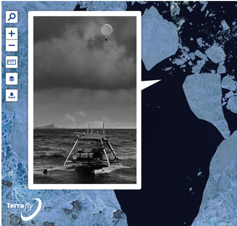
TerALTA balloon-mounted bathymetry sensor operated via a robotic vessel for NSF IUCRC Compendium CAKE-MSS Modeling Sea Surge and Flooding using ALTA and TerraFly. Image provided by CAKE.
